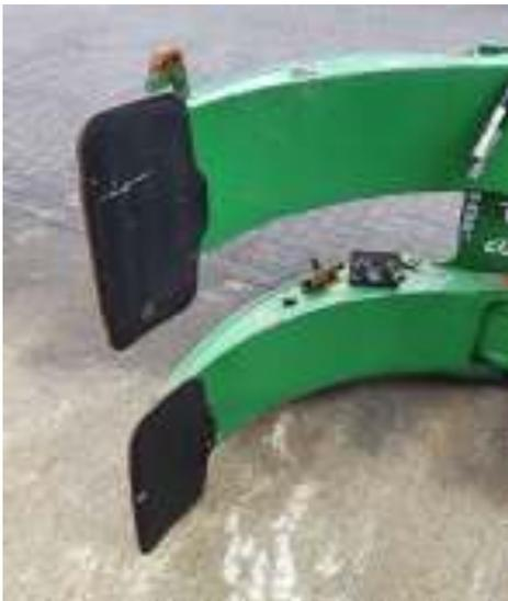
A growing number of machine breakdowns for the customer had led them to question the quality of their existing gripper pads. After some investigation, it transpired that the rubber covering for the pads was not up to a high standard resulting in significant disruption to their manufacturing processes.
